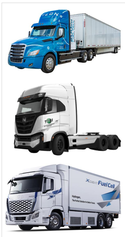
Figure 26. Overview of the fuel cell electric trucks available at the end of 2022 in the state of California under the HVIP Program. Top vehicle: Hyzon Motors HyHD8 FCET; Middle vehicle: Nikola TRE FCET; Bottom vehicle: Hyundai Xcient FCET. Source: Hydrogen and Fuel Cell Partnership, https://h2fcp.org/ (Accessed on: August 1, 2023).
