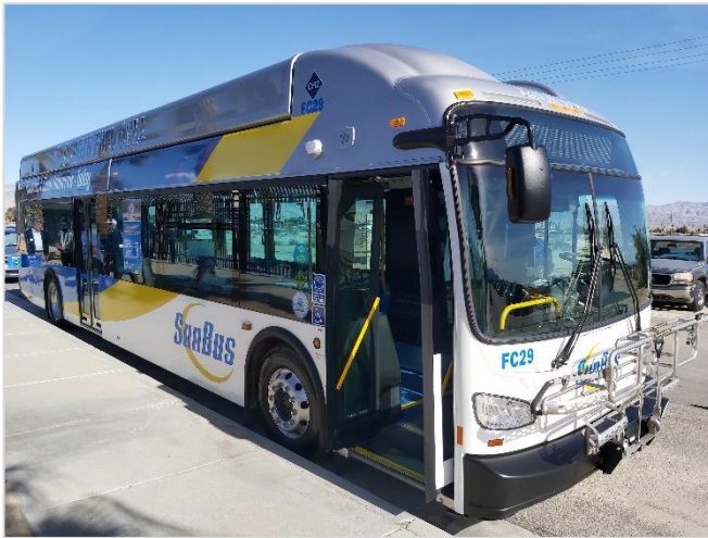
Figure 25. The New Flyer Xcelsior XHE40 FCEB deployed by SunLine Transit Agency. Source: Own resources from the author's study visit in the Sunline Depot in Thousands Palms, CA (January 14, 2023).
